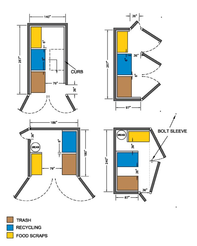
ALL FIGURES INCLUDE TWO 4 CUBIC YARD DUMPSTERS AND ONE 2 CUBIC YARD DUMPSTER. GREASE BARREL MEASURES 36" IN DIAMETER. DIMENSIONS TO INSIDE WALLS.
