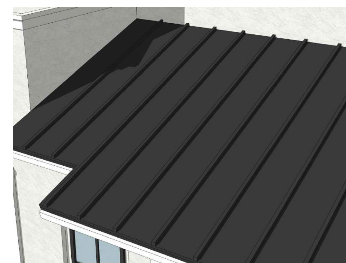
11 STANDING SEAM ROOF
