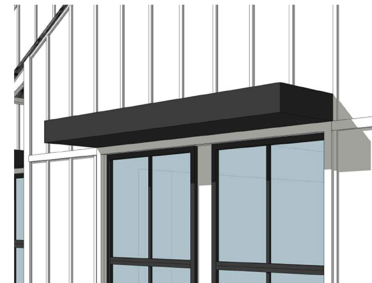
4 METAL AWNING OVER WINDOW
