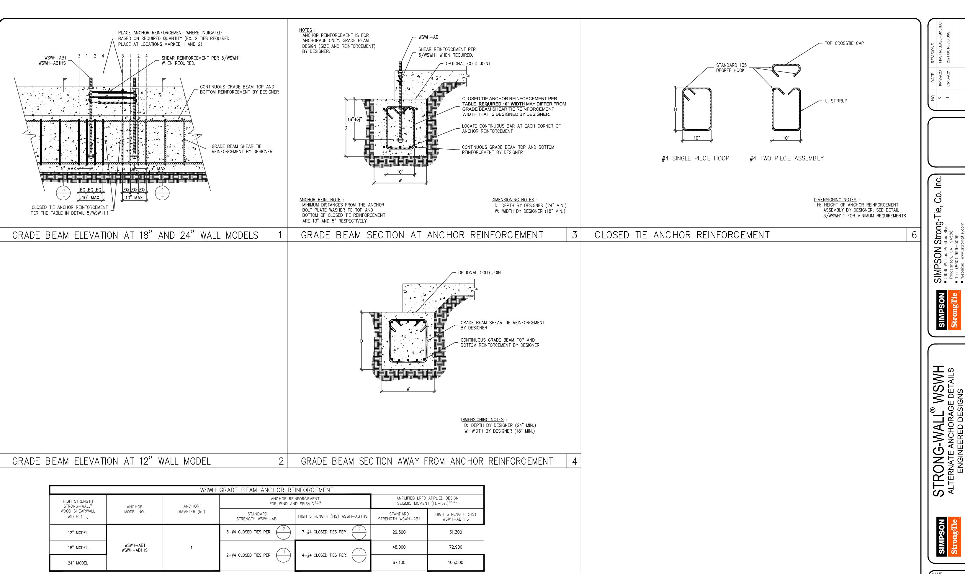
1. ANCHOR REINFORCEMENT CONFORMS TO ACI 318-19 SECTION 17.5.2.1, ACI 318-14 SECTION 17.4.2.9 AND ACI 318-11 SECTION D.5.2.9. FULL-SCALE TESTING WAS USED TO VALIDATE ANCHOR REINFORCEMENT
