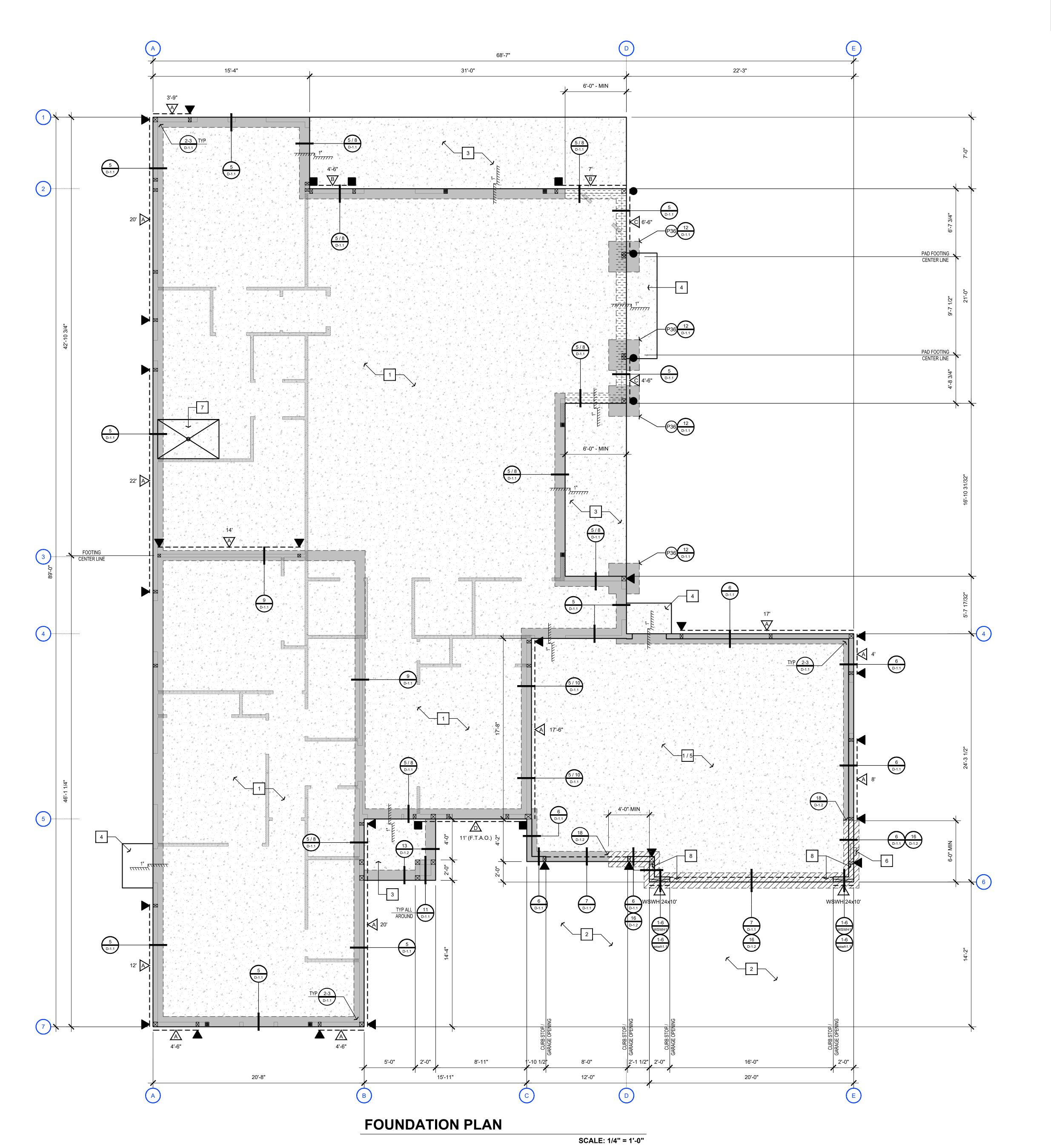
FEET OF COMPACTED SOILS BELOW THE BOTTOM OF ALL FOOTINGS. AREA OUTSIDE THE BUILDING AREA TO RECEIVE FILL, EXTERIOR SLABS-ON-GRADE, SIDEWALKS AND PAVING SHOULD BE OVER-EXCAVATED TO A DEPTH OF ONE (1) FOOT. THE EXPOSED SURFACE SHOULD BE SCARIFIED, MOISTURE CONDITIONED
