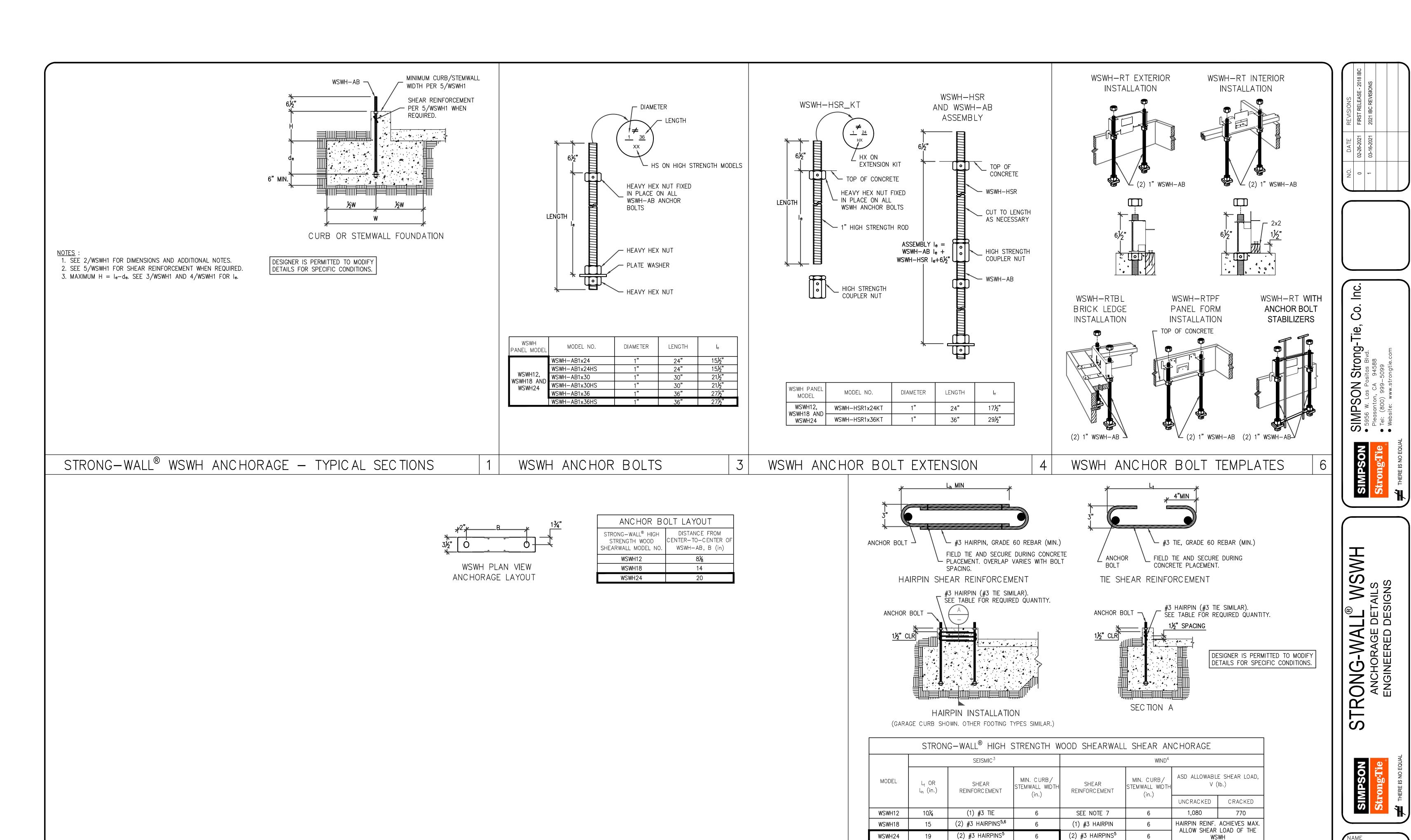
STRONG-WALL® HIGH STRENGTH WOOD SHEARWALL TENSION ANCHORAGE SCHEDULE 2,500, 3,000 AND 4,500 PSI
