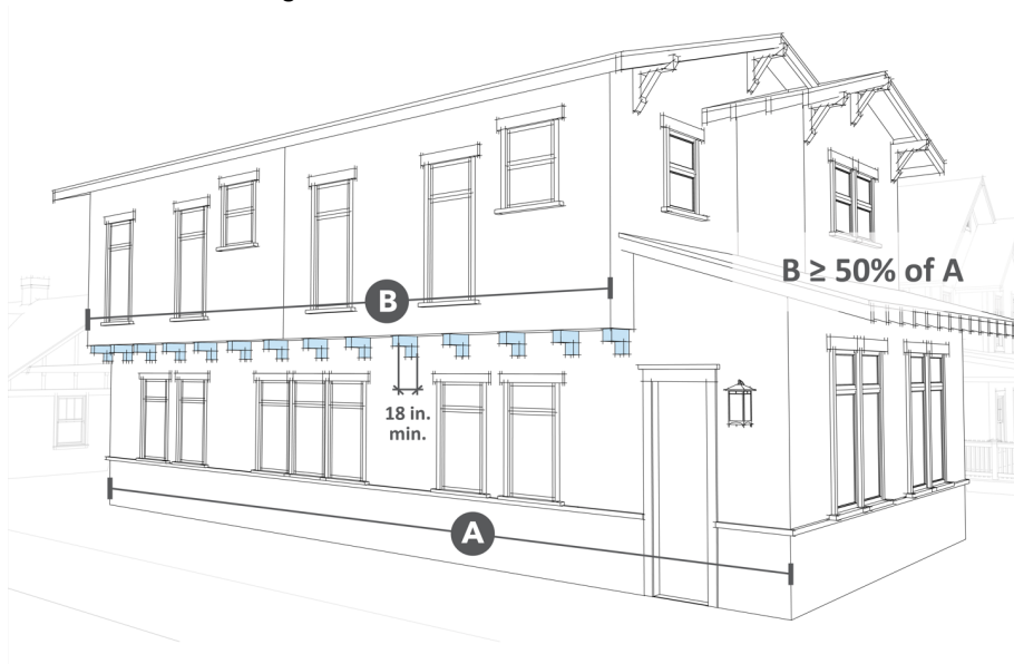
Figure 21.50.050-6: Corbeled End Beams
