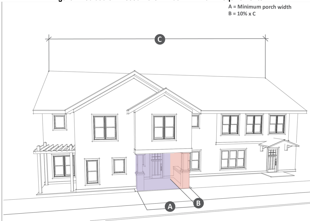
Figure 21.50.050-8: Exceed Porch Width Minimum Requirements
