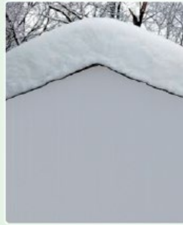
Durable Insulated Steel Roof, Snow Load Test of 30 lbs/sqft
