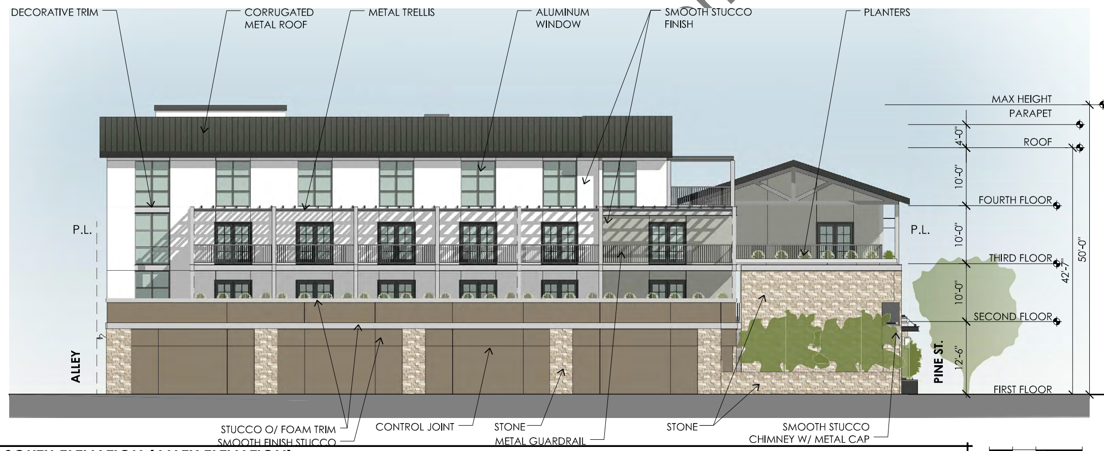
SOUTH ELEVATION (ALLEY ELEVATION)
