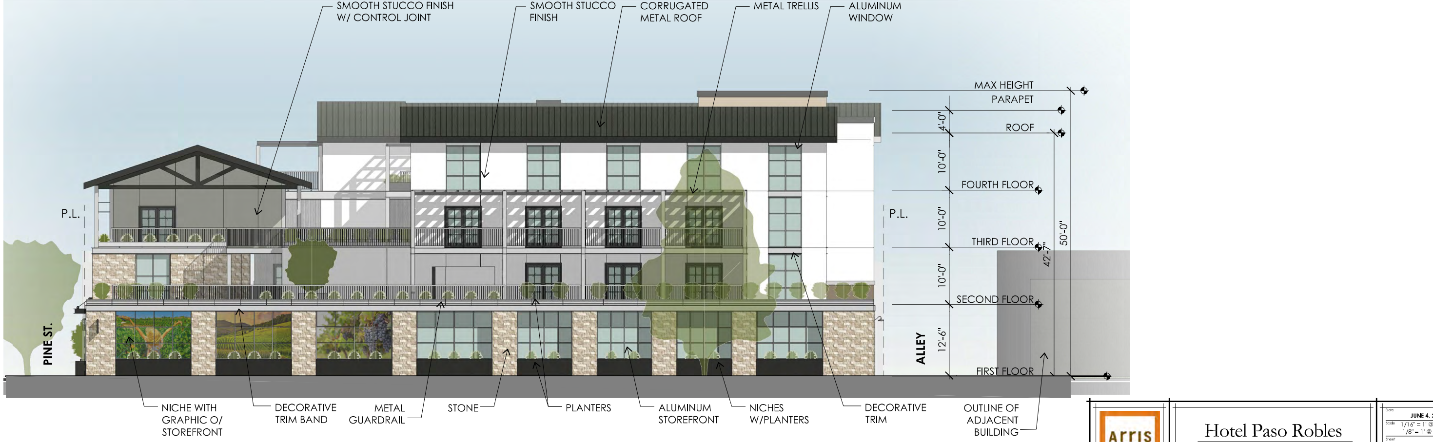
SOUTH ELEVATION (14TH STREET ELEVATION)
