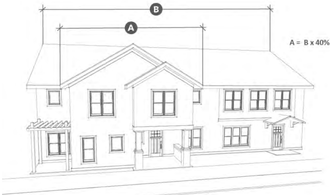
Figure 21.50.050-9: Gabled Roof Profile
