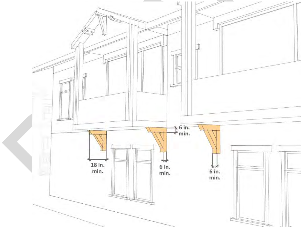
Figure 21.50.050-7: Post and Beam Supports
