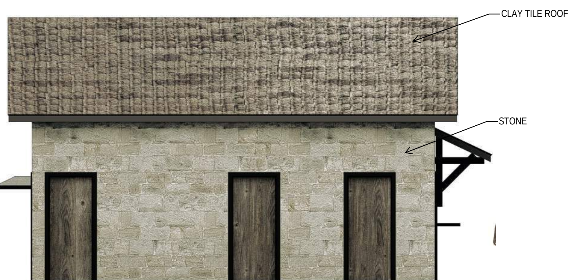
POOL OUTBUILDING - LEFT ELEVATION
