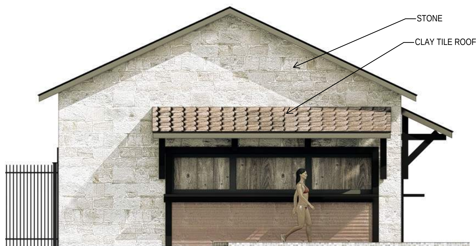
POOL OUTBUILDING - FRONT ELEVATION
