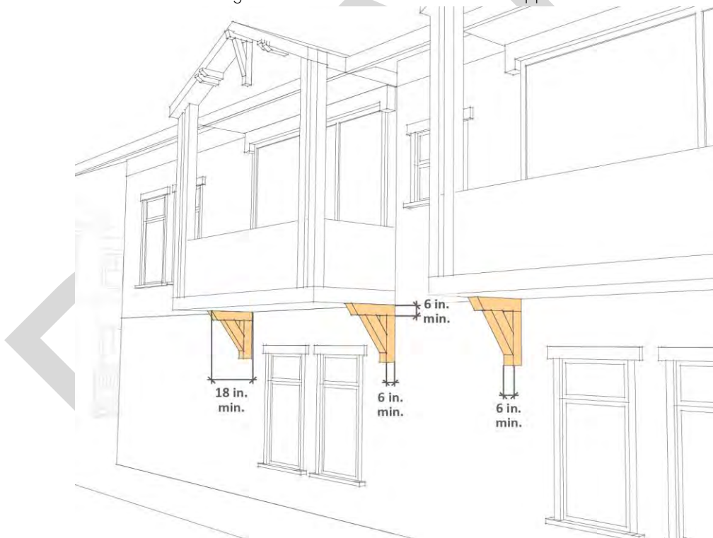
Figure 21.50.050-7: Post and Beam Supports
