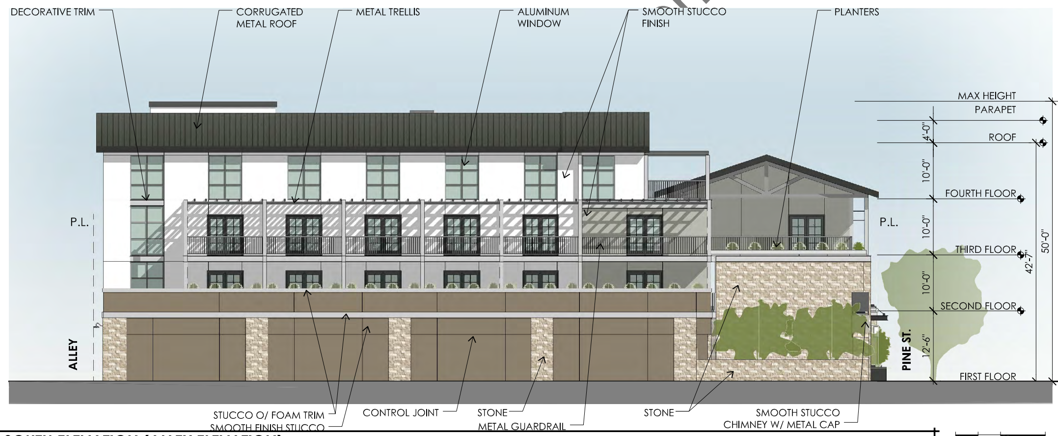
SOUTH ELEVATION (ALLEY ELEVATION)
