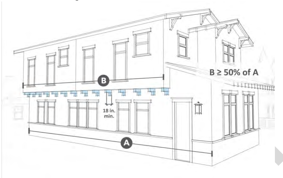
Figure 21.50.050-6: Corbeled End Beams
