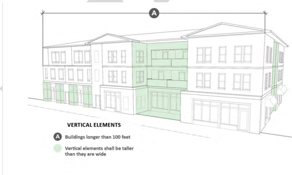
Figure 21.50.050-4: Vertical Elements on Horizontal Buildings
