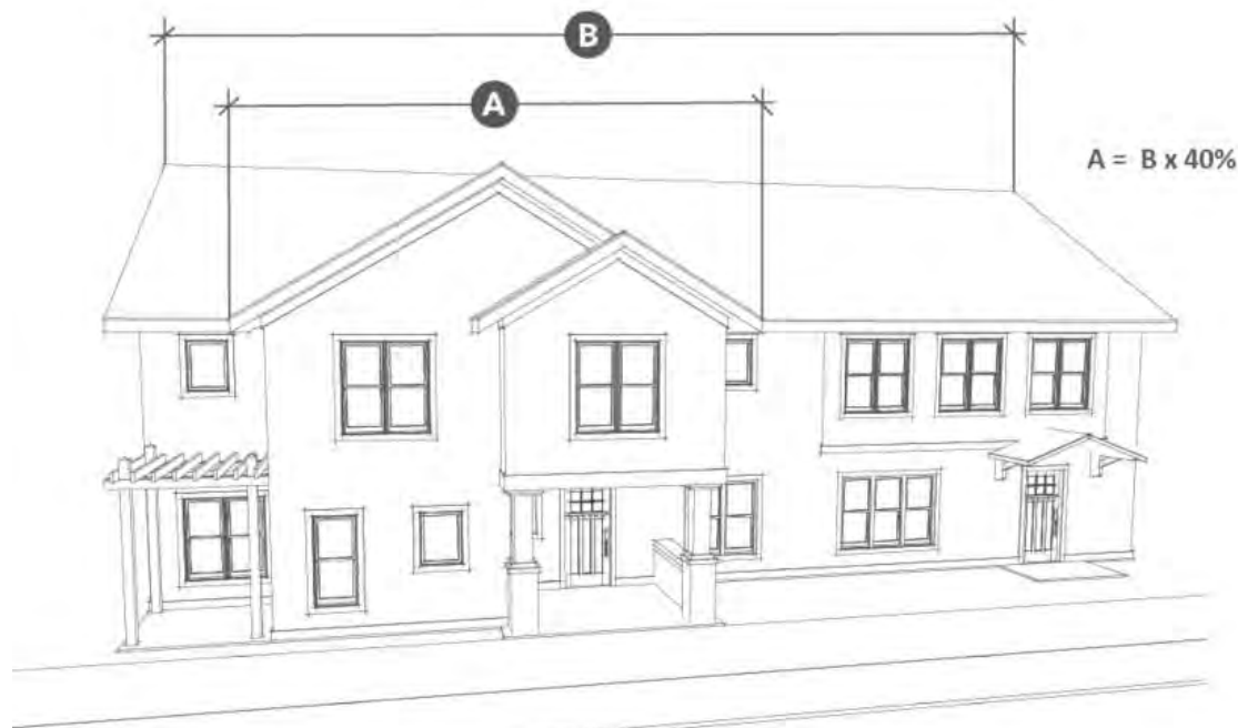
Figure 21.50.050-9: Gabled Roof Profile
